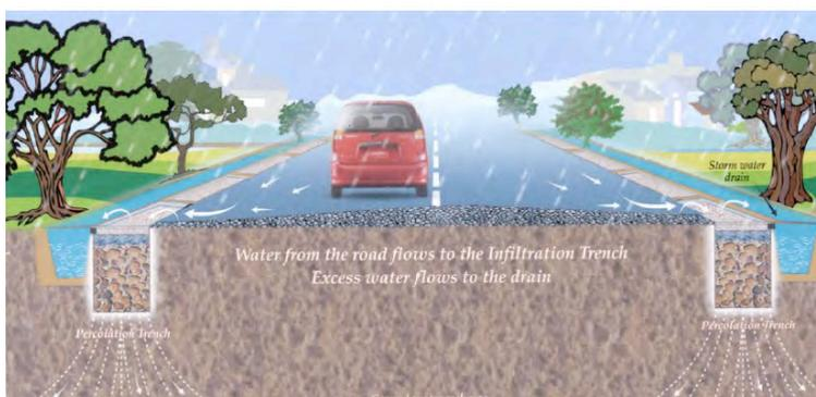
Here roads are built in such a way as to facilitate rainwater collection and ground water recharge through road-side trenches. They are about 600mm wide and 600mm depth, filled with pebbles /aggregates with a top layer of coarse sand.
